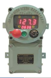
The POLMON "Integrated RPM Control" has been specially developed with integration of Temperature, RPM Measurement & RPM drive selection output to interface to VFD for agitator control in Pharmaceutical industry. It eliminates multiple devices mounting near the reactor which increases reliability and easy operation Software Calibration eliminates instrument opening in restricted areas.
