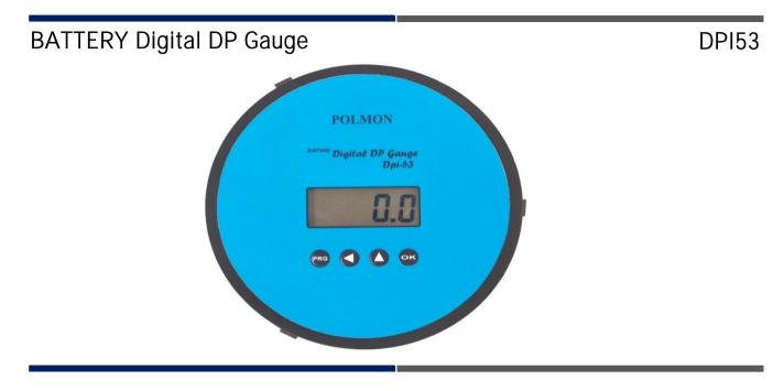
Digital DP Gauge (Model.No.DPI-53) is designed to measure difference between two pressures in Clean Rooms replacing the conventional Analog Gauge to eliminate the inherent problems. Operates with AA, Duracell, 1.5V, 4 No's batteries and a minimum of 18 Months Battery life with 1 Sec update Rate
