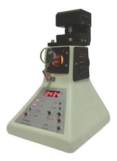
MP – 96 Digital Melting Point Apparatus is an ideal instrument for determining the characteristics / purity of materials based on Melting Point.
