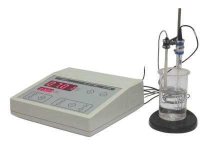
Microprocessor based TABLETOP LP-135M is an ideal instrument for lab. It can be used for measurement of pH, temperature, and mV. It incorporates Offset Slope, Calibration & Inbuilt temperature compensation. It is designed as the most convenient and user-friendly instrument considering practical problems while measuring pH. Easy operation with front panel keys.
