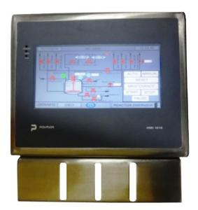
The POLMON "FLP HMI1010" Human Machine Interface designed to meet the requirements of operator interface to Industrial Control systems like PLC/DCS and other Ethernet devices or MODBUS devices on MODBUS RTU. It is specially designed for life science industries and suitable for use in Zone1, Zone2 Gas Gr.IIA & IIB Hazardous Area.
