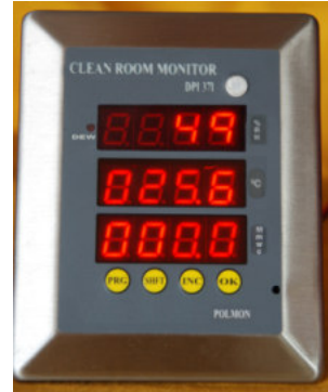
DPI37I with Inbuilt Sensors
